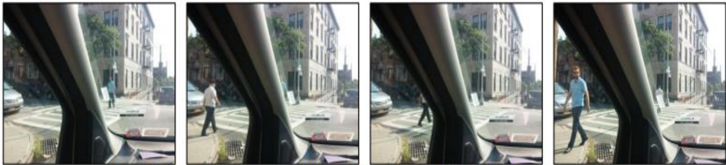
Pedestrians in the crosswalk can disappear behind the vehicle's A-pillar
