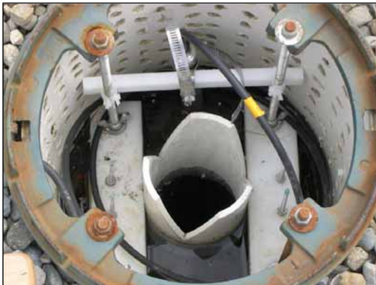
Figure 2-8 Installation of the V-notch Weirs for Monitoring Bypass Flows in the Roof Drain
