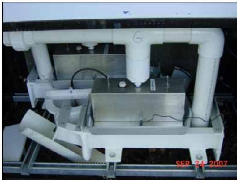
Figure 2-14 Two-Stage Flow Monitoring System (Tipping Bucket Coupled With HS-Flume)
