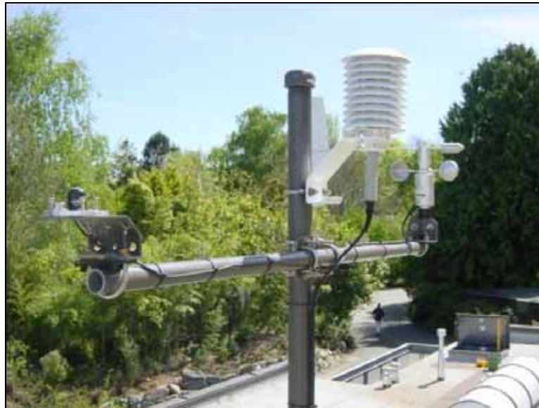
Figure 2-5 Weather Station Containing Wind Speed, Air Temperature, Relative Humidity and Solar Radiation Sensors
