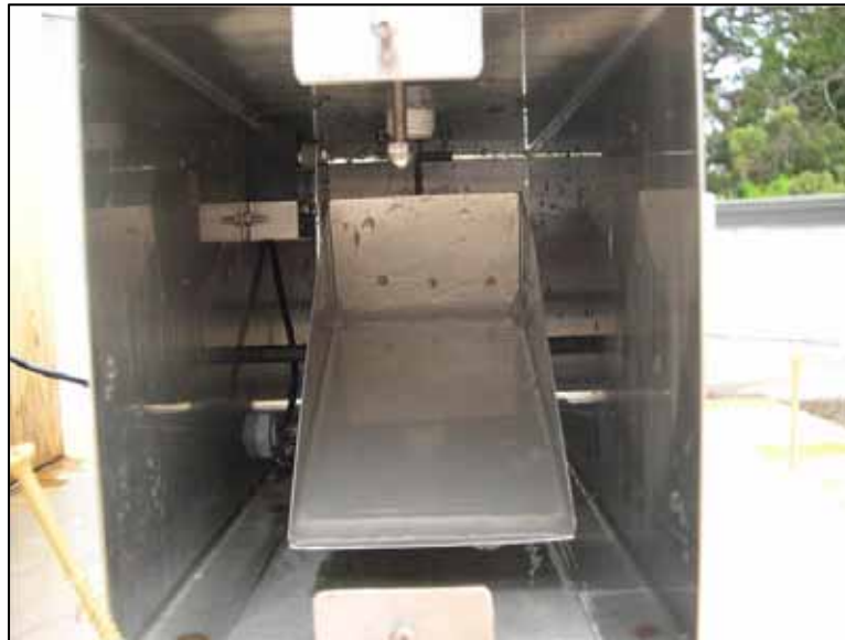
Figure 2-4 Unidata 6506H Tipping Bucket Flow Meter
