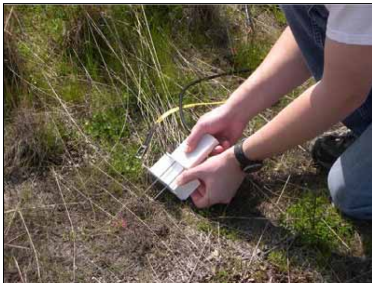
Figure 2-9 Installation of Soil Moisture Content Probe
