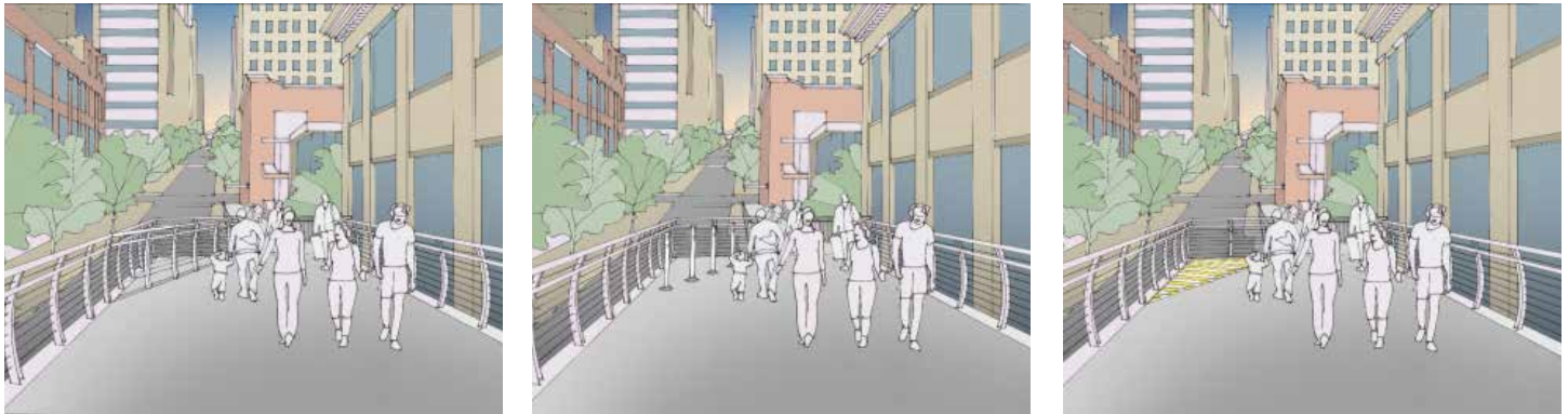
Figure 5: Temporary transition designs - railing (left), bollards (center), and pavement marking (right)
