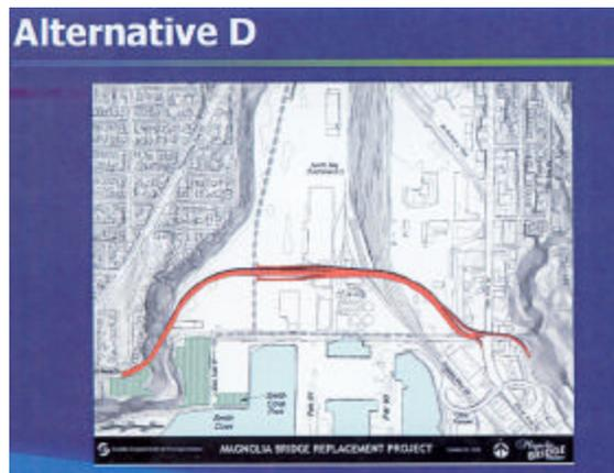
Alternative D – Construct a new bridge in the form of an arc to the north of the existing bridge.
