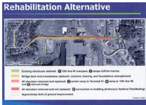
Rehabilitation Alternative – Bring the existing bridge up to current load and design standards using the existing bridge structure to the extent possible. Replace the bridge deck (roadway) and stabilize the foundation and concrete columns.
